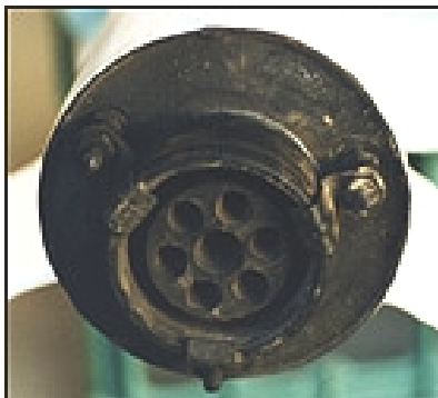
High temperature can cause roasting of the "business end"
