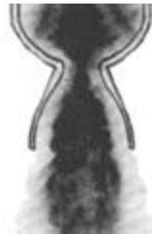
Exit area restricted by aft closure and nozzle, gases escape at supersonic velocity
