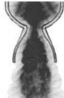
Exit area restricted by aft closure and nozzle, gases escape at supersonic velocity
