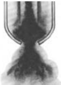
Exit area is restricted by aft closure, gases at acoustic velocity.
